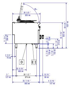
Cold Water inlet 1 (cleaning) D Drain FΙ Electrical inlet (power) HWI Hot water inlet
